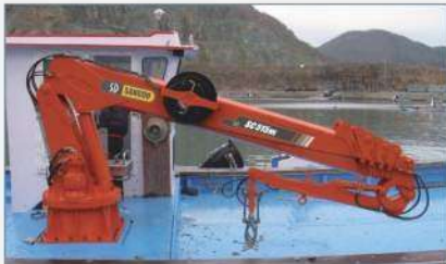
Pedestal Crane in Vessel
